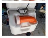
This example of adding a vent provides a low cost, low impact solution and can be applied to all types of toilets cassettes and waterless toilets. Due to the minimal size of the vent hose no additional exterior protection device fittings such as a vent cover or grill (reg 20, c, iii) will be required.
