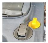
Some Thetford brand toilets have a fitted vent system that opens when the cassette is installed. These vent internally into the locker space or into a vent pipe / hose (image on right). The vents equalise pressure and release some gases/odour. The locker can then be easily vented to the exterior of the vehicle.
