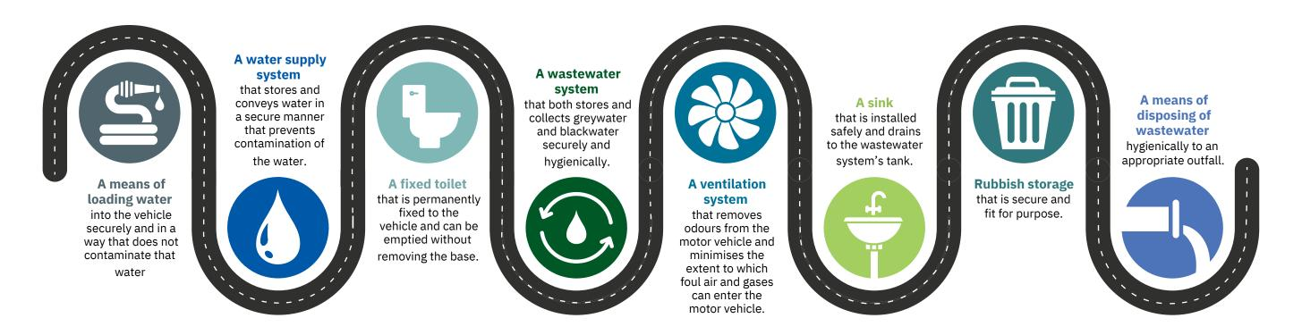
Each of these facilities must be able to be used for at least three days for the maximum number of people the vehicle is certified for. Facilities must be fit for purpose and properly installed.
